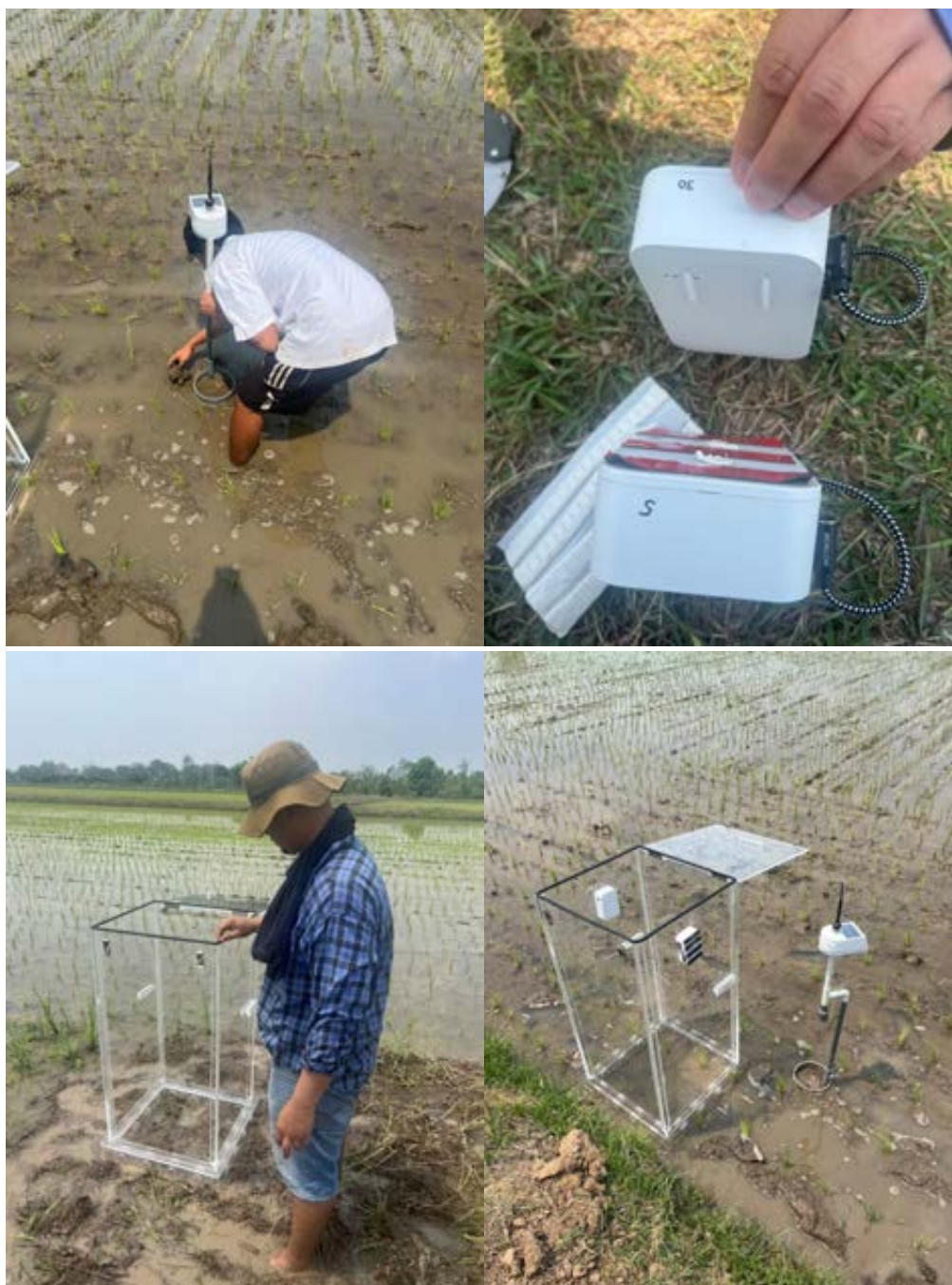
Figure-2. The figure depicts the setup within the RID paddy field in Nakhon Pathon, showcasing \text{CH}_4 methane emission measurement equipment, accompanied by a closed chamber and sensors for monitoring water levels.
