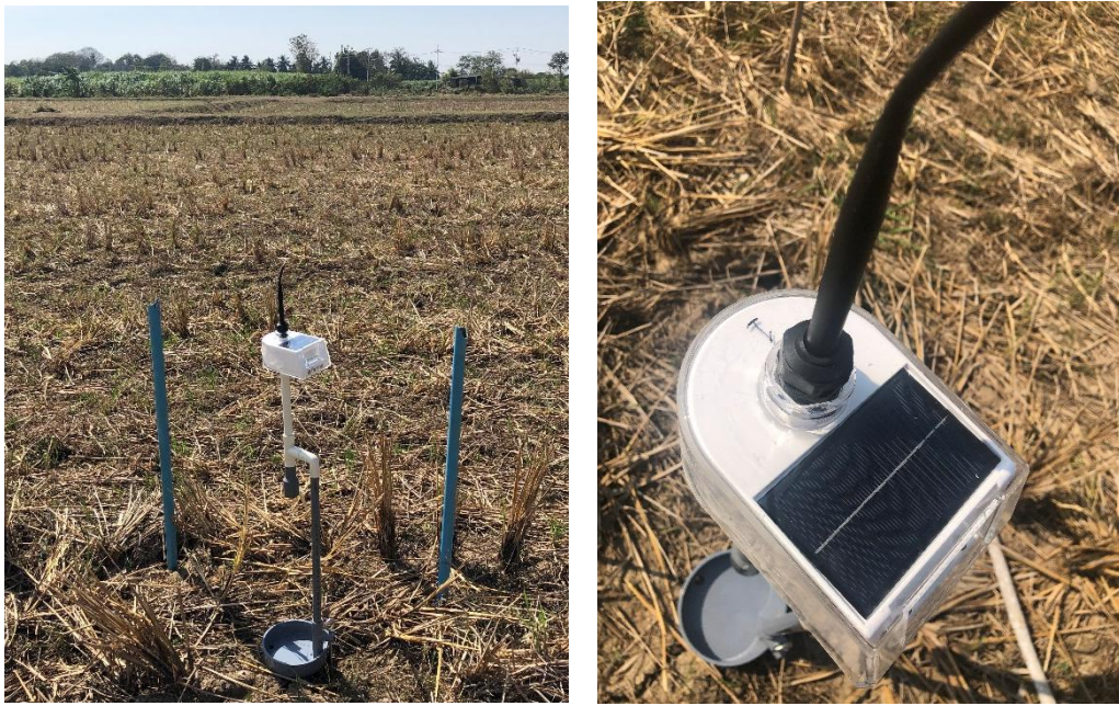
Figure-1. Solar-powered Farmo water level sensors in RID paddy field
