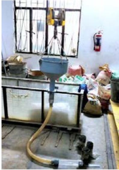
Figure 3: Portable pluviator for construction of the model wall
